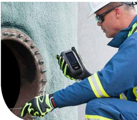
*With an internal pump that's always running, the Honeywell BW™ Ultra pulls air through a sampling hose and assesses it for gas hazards, giving you an easy-to-read picture of safety.*
